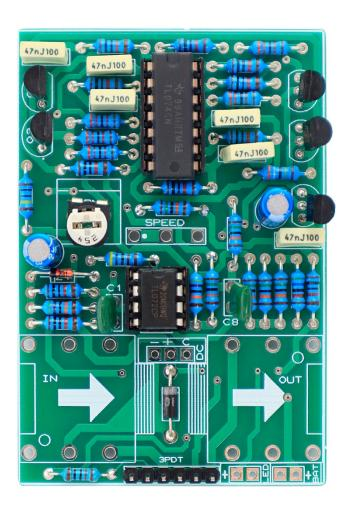
Solder the capacitors and transistors. If you have troubles reading the values, check out our <u>"Reading Part Values"</u> tutorial. Pay attention to the orientation, as well as to the polarity for electrolytic capacitors.
