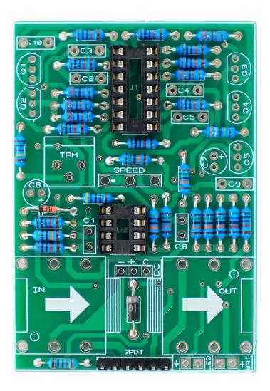
First of all place the IC sockets (without the ICs). Pay attention to the orientation! The small notch in the socket should be oriented as indicated in the PCB.
