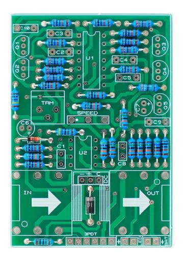
Place the resistors and diodes. If you have troubles reading the values, check out our "Reading Part Values" tutorial.
